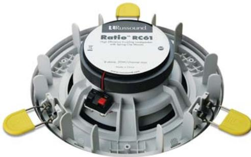
To benefit installers, Russound developed spring-clip locking retainers that reduce installation time. In-ceiling speakers are simply pressed into the cutout, enabling the clips to snap into place and secure the speaker. For the in-wall model, the spring clips hold the speaker in the wall, making it easier to square up the speaker while tightening the dogleg grips.
